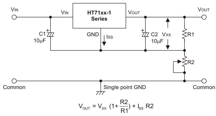
**Circuit for Increasing Output Voltage**
